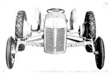
Caution: Loosen the bolt through the radius rod yoke first, then spread axle as desired. No change in the steering connection is necessary. Always assemble the axle with one hole between the bolts holding the halves together, never in adjacent holes.
