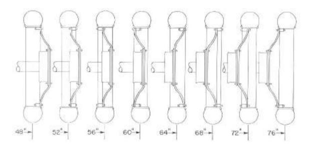
Treads of 48, 52, 64, 68 inches are made without changing rear wheels to opposite side of tractor. Treads of 56, 60, 72, 76 inches are made with rear wheels changed to opposite side of tractor, to keep treads running the proper direction. Note: Arrow on sidewall of tire must always point in direction of travel.
