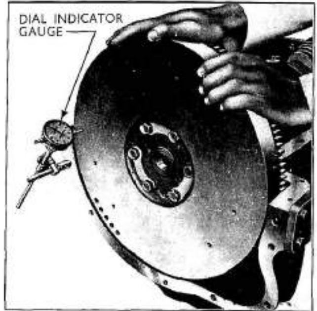
Fig. 45 Testing Flywheel Run-out
