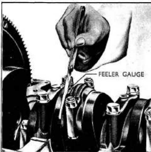
Fig. 25 Checking Connecting Rod End-float
