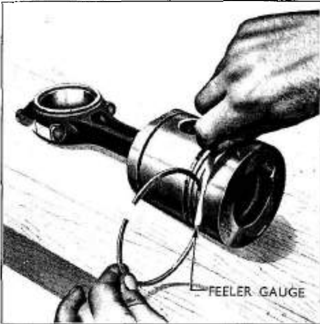
Fig. 23 Checking Ring to Groove Clearance
