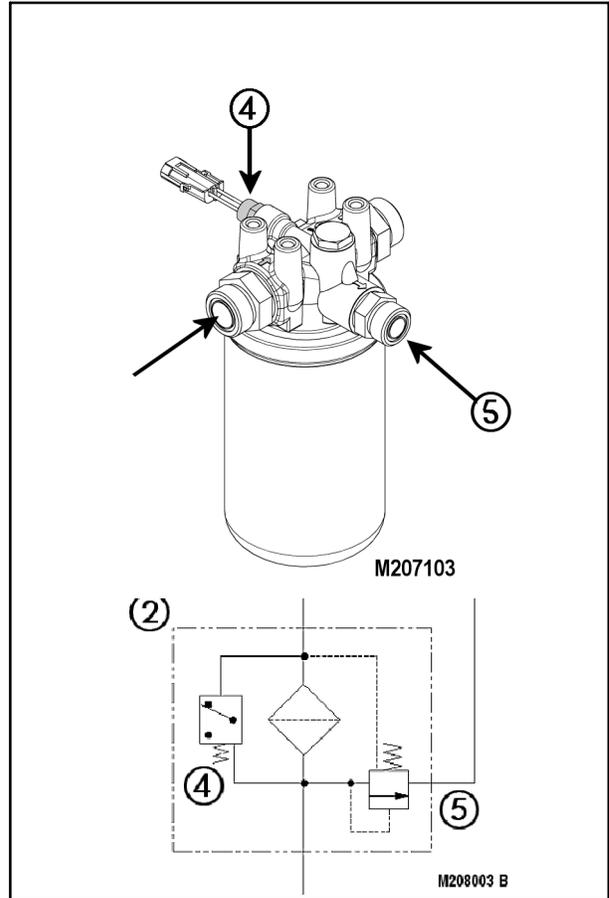
**Control / Lubrication Pressure Valve**
