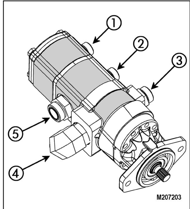
**NOTE:** If the seal was to leak between the front and center pumps oil could transfer between reservoirs.
