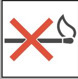
**⚠ WARNING** Fire or explosion possible. Fumes could ignite and cause burns. No smoking, no flame, no spark. 275-419 (2P)
