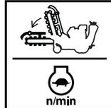
**⚠ CAUTION** Tip over possible. When loading/unloading run at low idle and keep boom low. 270-7596
