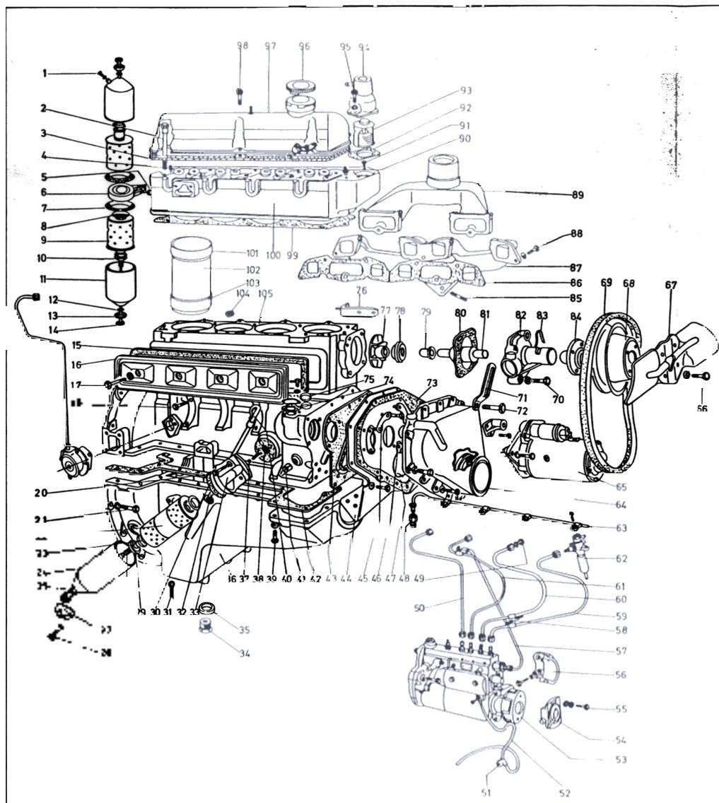
Fig. 01A-01-01 - Despiece del motor 2890
