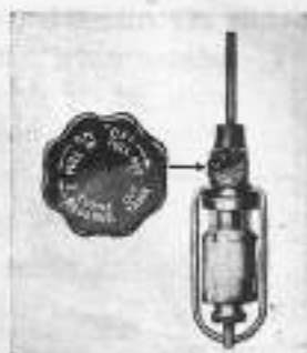
Sediment bowl with reserve fuel control. Remove bowl and filter and clean every week.
