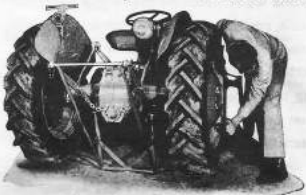
Adjusting rear wheel tread width. Note use of Ferguson Power Jack.
