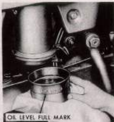
Figure 21 Checking the Air Cleaner Oil Level
