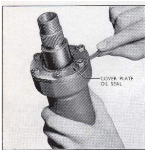
Fig. 11 Steering Main Nut Bearing Adjustment
