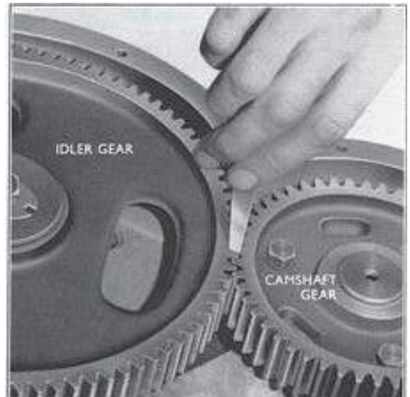
Fig. 9 Checking Timing Gear Backlash
