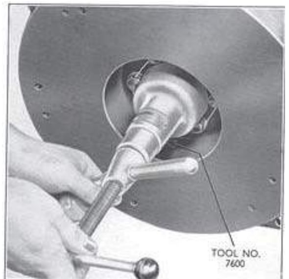
Fig. 19 Removing Clutch Pilot Bearing
