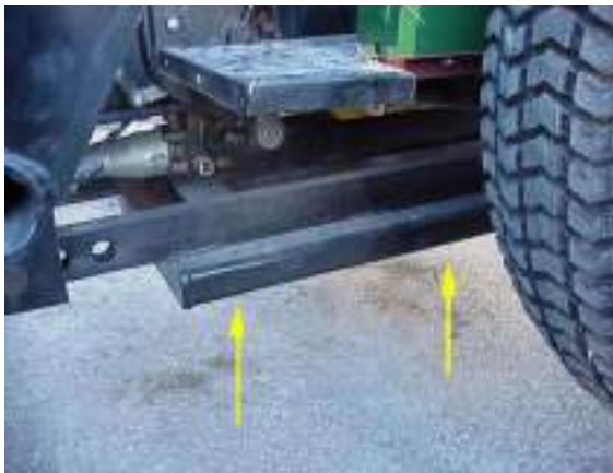
Figure 40. Hoe Frame showing heavy reinforcement
