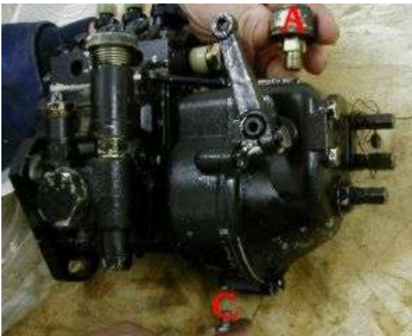
Figure 29. Fuel Injector Oil filler (A) & Drain (C)
