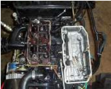
Figure 20. JM204 TY29 Engine with valve cover removed
