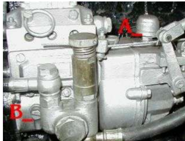
Figure 30. Fuel Injector Breather (A) and Cap (B)
