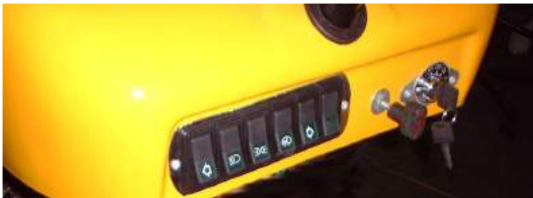
Figure 14. New style lower dash switches
