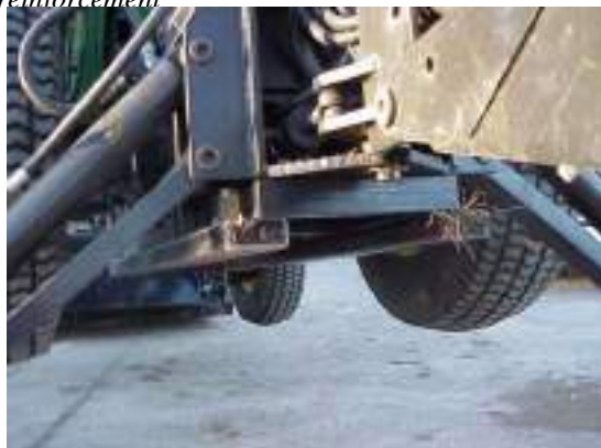
Figure 42. Hoe frame reinforcement fwd view
