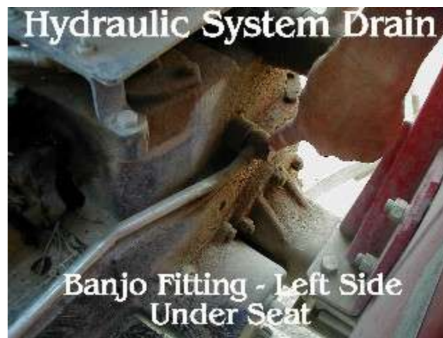
Figure 35. Hydraulic System Oil Drain
