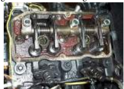
Figure 21. Close-up of JM-204 TY290 engine head
