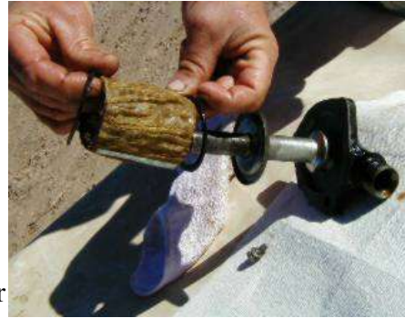
Figure 25. Hydraulic filter disassembly
