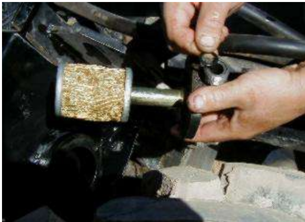
Figure 28. Hoe Hydraulic Filter o-ring
