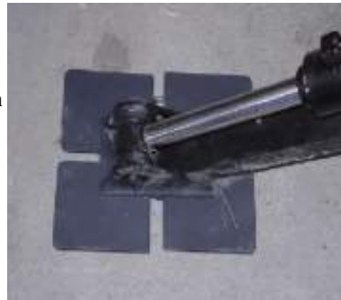
Figure 39. Enlarged Outrigger Pads
