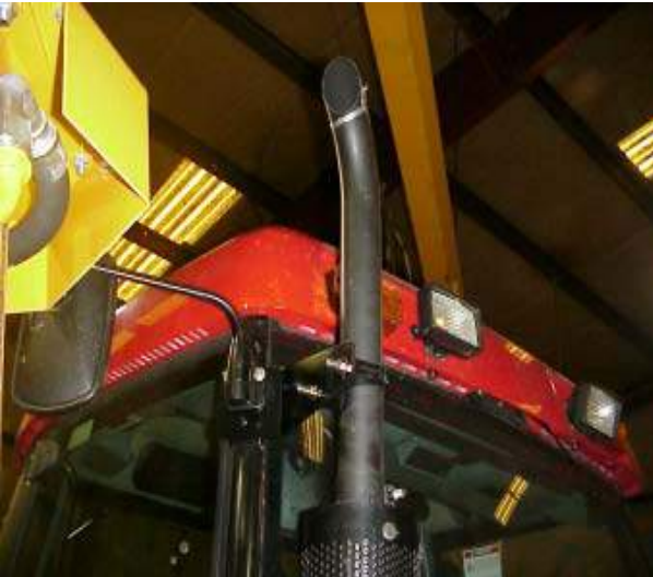
Exhaust Moved Inward Approx 9"
