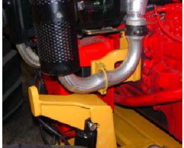
Replacement Exhaust Pipe Installed
