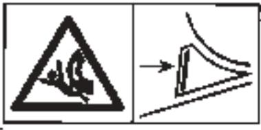
Before parking the machine, secure it with wheel chocks against unintended rolling.
