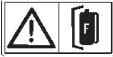
The machine may be taken into operation only when a suitable fire extinguisher is at hand.
