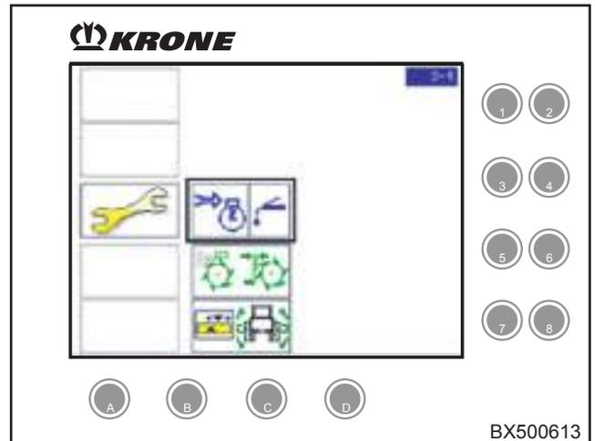
The display shows the „Clean central lubrication“ mask.
