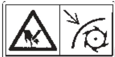
While performing grinding work, keep your distance. Close the protective cover once you have completed the grinding work.
