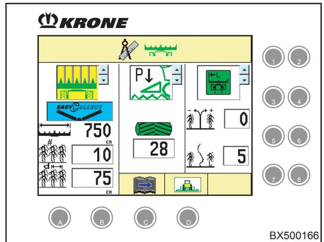
**4.6.2.2 Setting the maize header working width**
