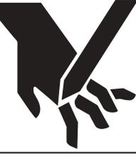
Avoid bodily injuries from rotating knives. Keep hands out of knife area when cutter head is turning.
