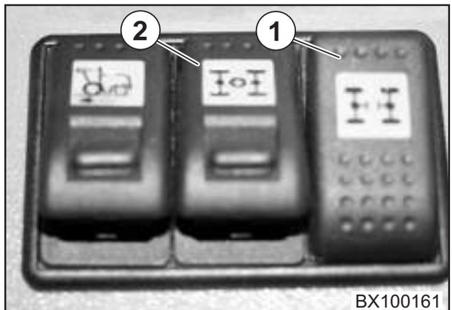
When all-wheel drive is switched off, axle separation is also switched off.
