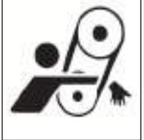
Components behind guards or access doors in this area may rotate several minutes after power is shut off.
