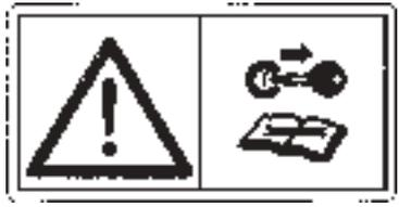
Before performing maintenance and repair work, switch off the engine and remove the ignition key.
