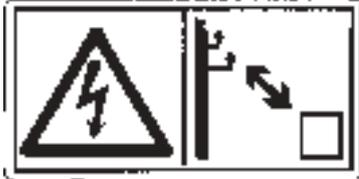
Keep the stipulated safe distance to power transmission lines.
