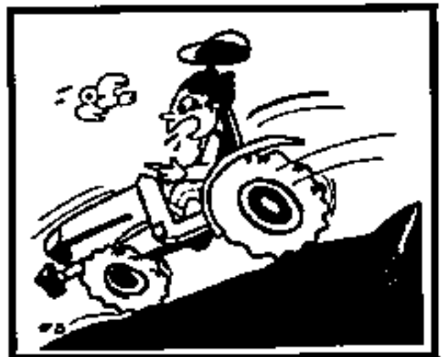
Be at a slow, controlled speed going downhill. Do not take your tractor up or down steep inclines.
