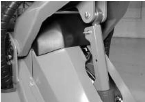
Make sure to secure the service support by locking it on the piston rod by the bolt
