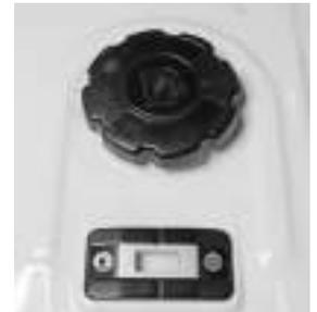
**Diesel engine:** Check fuel level and fill the tank if necessary. Use diesel fuel only, in accordance with the instructions in the Kubota engine Operator's Manual. Use of other fuels is not allowed, because their quality and properties cannot be guaranteed. Make sure not to let the fuel tank get empty. Should this happen, refuel and restart – the engine is fitted with automatic fuel bleeding.
