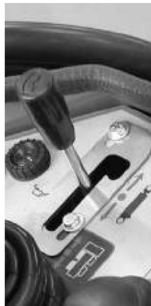
On model **320S+** auxiliary hydraulics are controlled with the lever no. 2 in the footwell left (see page 13).
