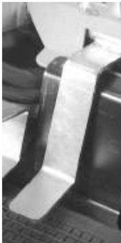
Models **313S**, **314S** and **320S** have a double speed function (optional extra) which is operated with a pedal in the footwell (see picture). Double speed can be engaged either before starting driving or while driving. It can also be disengaged at any time during driving or after the driving by lifting the foot off the pedal.
