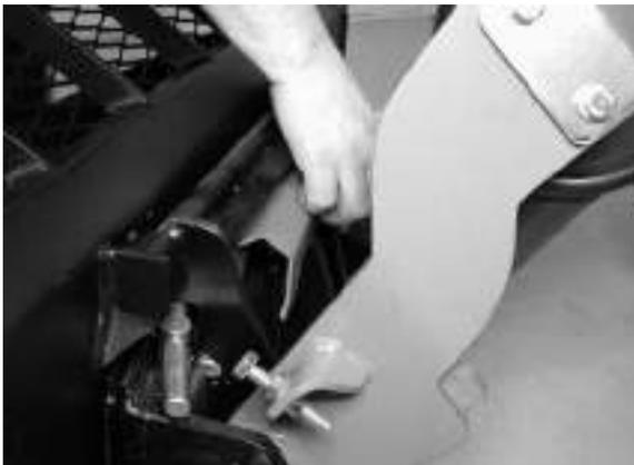
Hydraulic oil tank is located on the front axle as a part of the front chassis, so in order to get to the dipstick and return oil filter the boom must be lifted and the front cover plate removed.
