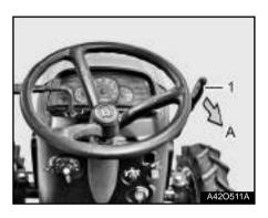
(1) Hand throttle lever (A) Engine rpm increases
