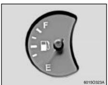
Check the fuel gauge. Make sure that a sufficient amount of fuel is in the tank
