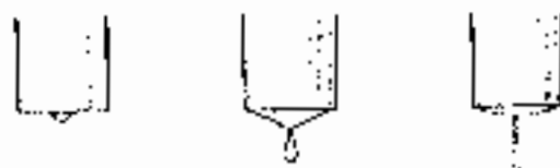
Good Bad Bad Dribbling in test condition
