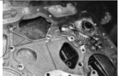
Fig 5-24 Lubricating Pipes Installation
