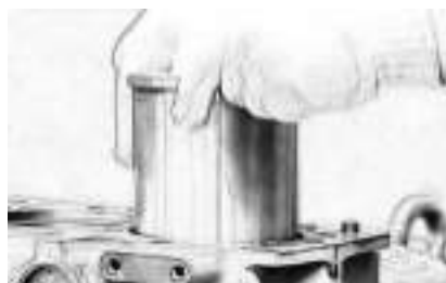
Fig 5-7 Wet Sleeves Installation
