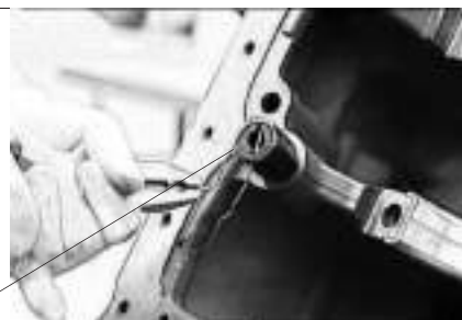
Fig 5-2 Pressure Limiting Valve of Oil Pump
