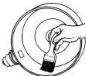
Fig 3-5 Clean Dust Accumulator
