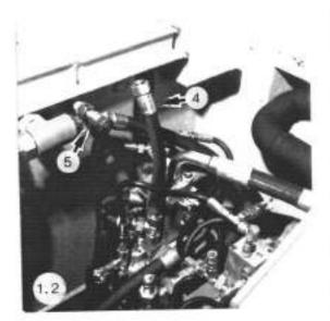
1.3 All valve caps must be bleed before starting up operation for the first time.
