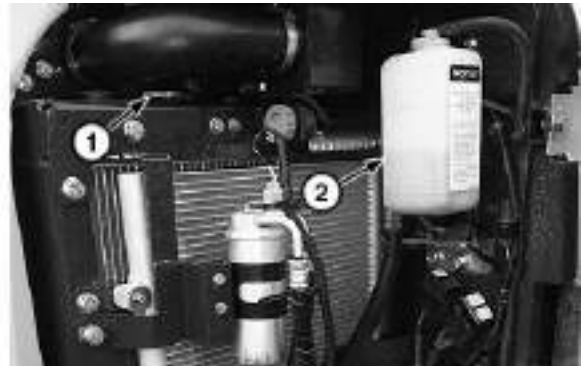
Coolant Recovery Tank
