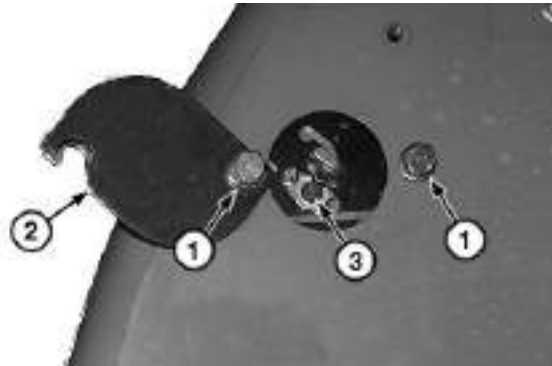
Fuel Tank Drain Valve
