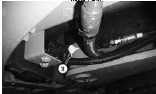
Radiator Drain Valve
