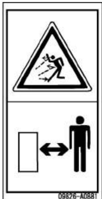
(15) Warning against spattering debris (09826-A0881)
