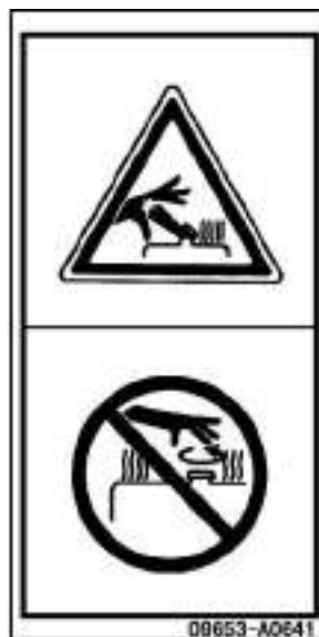
(6) Precautions for oil at high temperature (09653-A0641)
