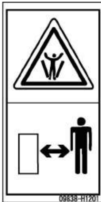
(14) Precautions when inspecting the crusher (09838-H1201)
