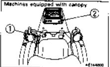
Place fuel control lever ① in the low idling position and run the engine at low idling speed for about 5 minutes to allow it to gradually cool down.
