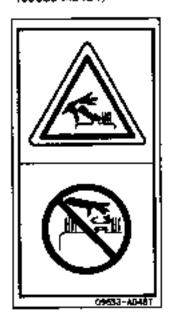
Never remove the cap when the angine is at operating (high) temperature. Stream or high temperature oil blowing up from the radiator or hydraulic tank, will cause personal injury and/or burns.
