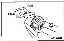
Check that the safety lock lever (§) is locked.
