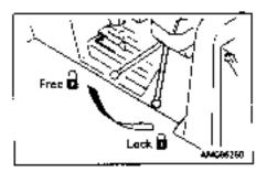
Operate blade control lever (§) to the LOWER position, and lower the blade to the ground.
