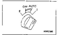
(2) When the preheating is completed, turn the key in starting switch ② to the START position to start the engine.
