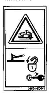
There is the hazard than machine may move suddenly and catch or run over someone near the machine causing injury.
