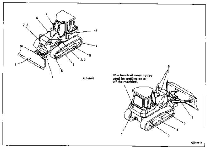
Check for demage, wear, play in work equipment, cyfinders, linkage, hoses
