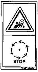
There is the hazard of being caught in the rotating parts of the machine causing injury.
