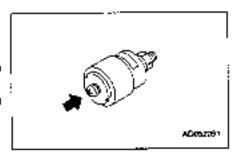
Replacing inner element
