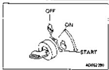
(3) After starting the engine, return glow switch ③ to the OFF [ position.
