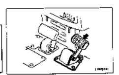
This pedal is used for reducing the engine speed or stopping the machine.
