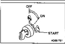
Remove the key from starting switch ②.
