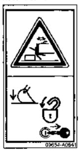
There is the hazard that machine may move suddenly and catch or run over someone near the machine causing injury.
