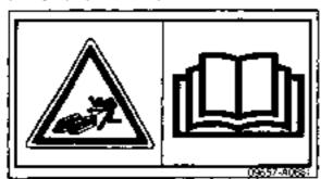
Plug coming from track shoe tension adjustment device causing injury. Read the operation and maintenance manual and carrying out the correct method when loosening track tension.
