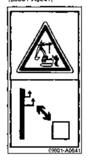
If machine goes close to high-voltage cables, it will result in electric shock to the operator.
