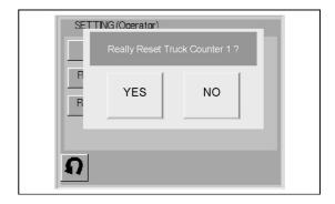
When this button (3) is pressed, the confirmation screen in the diagram on the right is displayed. Press the (YES) button. Count (B) for the previous operation on the dump counter screen is reset to 0.
