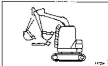
Set the work equipment in the posture shown in the diagram on the right, then operate the left offset and check that the work equipment automatically stops when it comes close to the operator's compartment.
