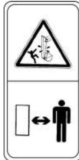
9. Falling from upper structure warning. This is located on the front of the fuel tank, on inside of walkway door, top of the counterweight.(20E-00-K1110)
