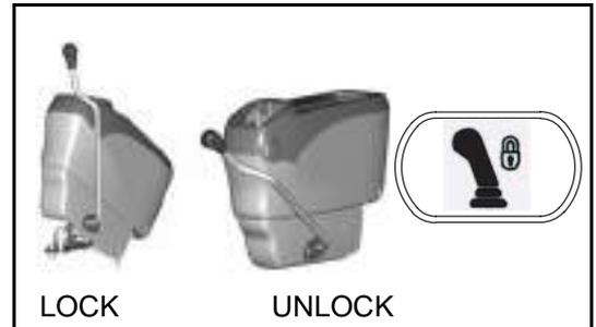
1. Before travelling on a Public Highway, with the safety lock lever lowered (in the UNLOCK position) engage the control lever lock switch to prevent accidental use of the work equipment, the rear brake lights will now become active.
