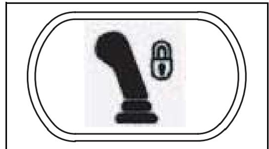
Before moving off, lock all machine cover and toolbox doors to prevent accidental opening.
