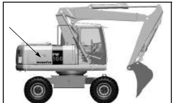
2. The refuelling pump is located in the compartment at the rear right hand side of the machine.
