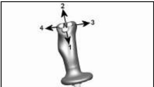
When the right control lever in this position, the boom and the bucket will be retained in the position in which they stop.
