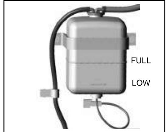
1. Open the rear door on the left side of the machine and check that the cooling water level is between the FULL and LOW marks on radiator reserve tank (1) (shown in the diagram on the right). If the water level is low, add water through the water filler of reserve tank to the FULL level.
