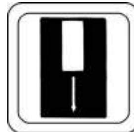
17. Travel Height -UK spec only. This is fitted to the top right hand corner of the front window (20E-00-K1720)
