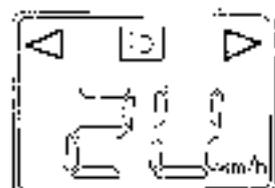
When the turn signal lamp flashes, the pilot lamp also flashes.
