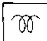
This lamp lights up when electrical heating circuit activates.
