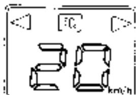
This meter indicates the running speed of the machine.
