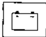
This monitor indicates an abnormality in the charging system while the engine is running.
