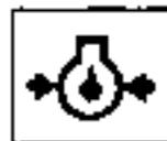
This monitor indicates a low engine oil pressure.
