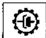
This lamp lights up when the transmission cut-off selector switch is turned to ON.
