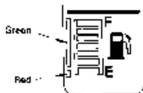
This gauge indicates the amount of fuel in the fuel tank. If there is enough fuel in the tank while the engine is running, the green range lights. If the red range lights, there is less than 36 liters of fuel in the tank.
