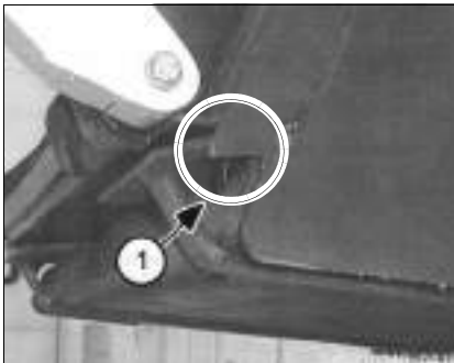
Fig. 132: Locking the attachment with the attachment adapter
