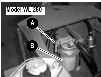
Fig. 135: Bleeding the fuel system
