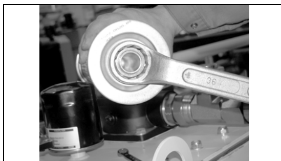
Figure 9.5 Open the filter assembly
