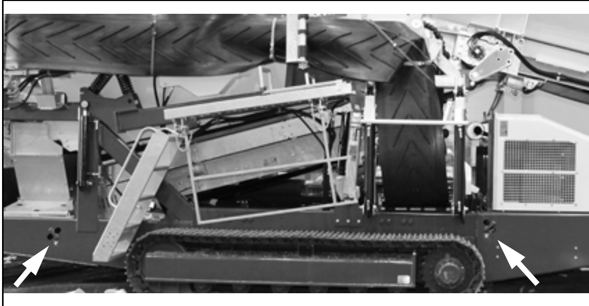
Figure 6.6 Fastening points of the unit
