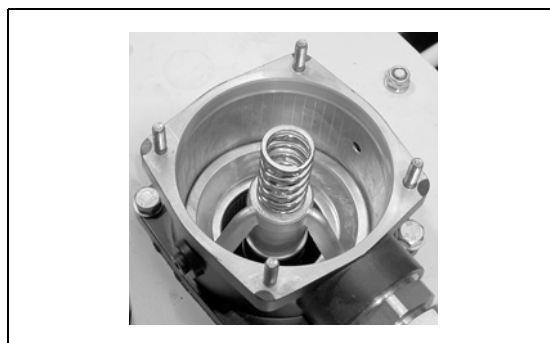
Figure 9.3 Undo the cover.
