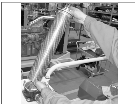
Figure 9.4 Remove the filter
