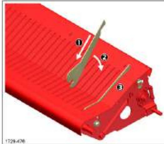
Figure 54. Replacing blank knives
