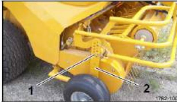
Figure 63. Pick-up gauge wheel
