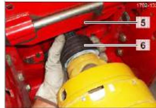
Figure 33. Driveline —couple to tractor
