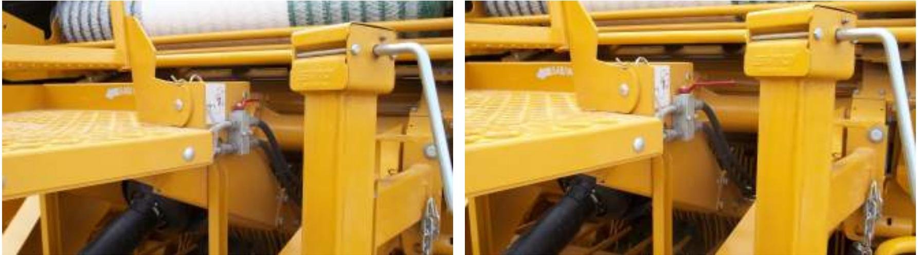
Figure 4. Tailgate hydraulic valve
