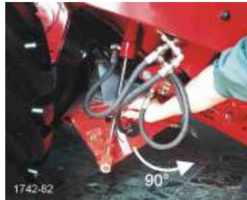
Figure 75. Knife axle lever
