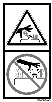
Fig. 18: Hydraulic oil tank under pressure
