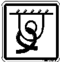
Fig. 6: Label for points used for strapping down the machine
