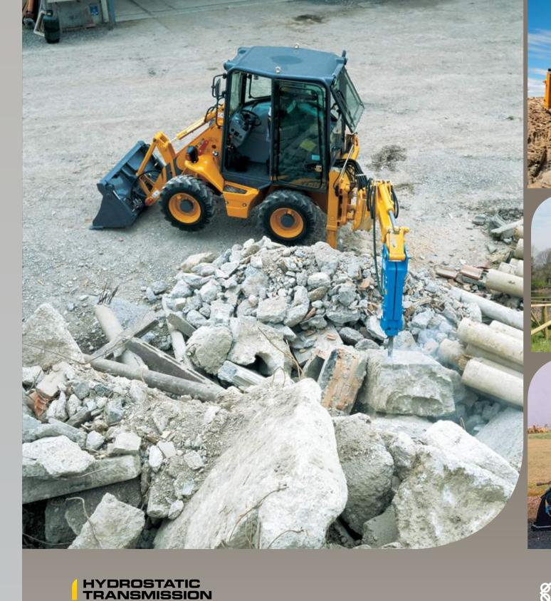
The hydrostatic transmission, joined with twin drive axles both equipped with 40% self-locking
