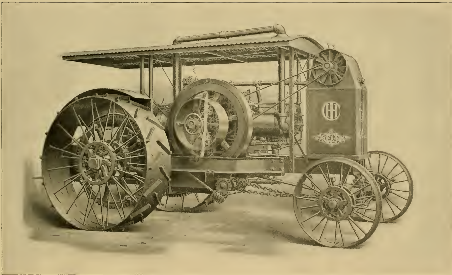
Right side view—15-H. P. opposed double cylinder I H C Mogul Gasoline Tractor
