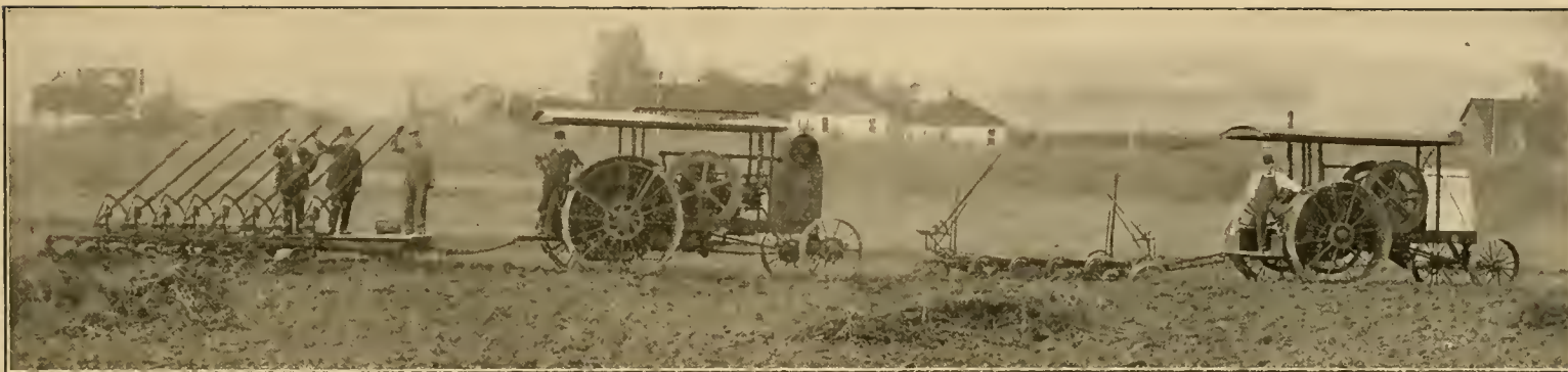
I H C Mogul 15-horse power tractor pulling an 8-furrow gang, and 20-horse power Mogul tractor pulling a 4-furrow gang
