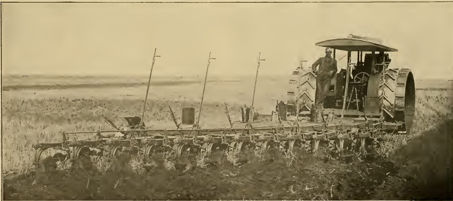
I H C Mogul 45-horse power tractor pulling a Case 12-furrow 14" breaker engine gang on the Elk Valley farm, Larimore, N. D. Conditions on this farm are such that the engine will handle a 12-furrow gang. Ordinarily, an 8-furrow gang is the largest plow which should be used with a tractor of 45 brake horse power
