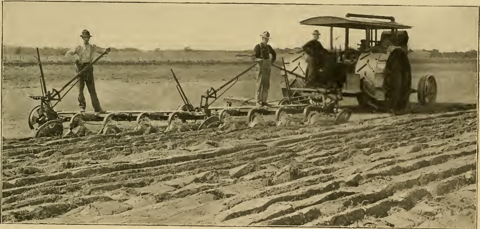
45-H. P. I H C Mogul Gasoline Tractor, owned by John McQueen, Kirkland, Ill., pulling two 4-furrow gangs Drive wheel equipped with 12-inch tire extensions
