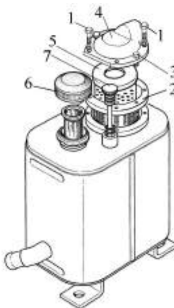
Fig. 8.4.40 – Replace filter element in HSU tank of BELARUS-1021.3 tractors
