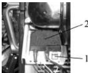
1 — fuse, 2 — voltage changer.
