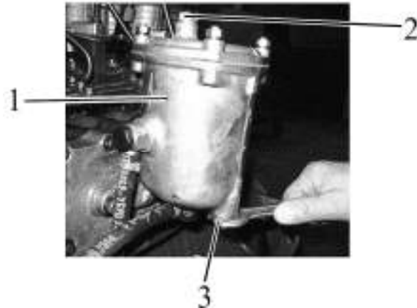
Figure 6.4.29 – Drainage of sediment from the fine fuel filter of diesel
