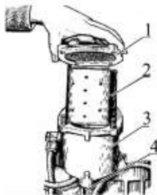
1 – filter cap; 2 – filter cartridge; 3 – filter housing; 4 – plug.
