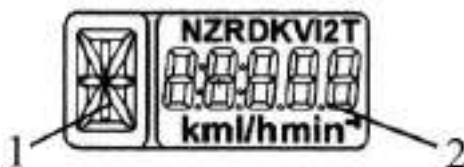
Figure 2.7.3 – Information fields of the multifunctional display
