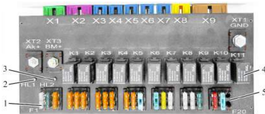
1 – cutout fuse; 2, 3 – signal led lamp of yellow color; 4 – electromagnet relay; 5 – signal led lamp of red color.
