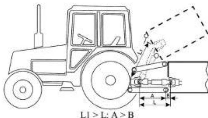
Figure 5.7.2 – Cardan shaft length finding scheme in course of the tractor coupling with the implements connected via RLL and FLL.
