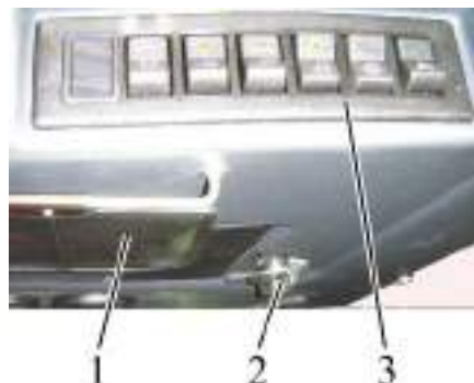
1 – sun visor, 2 – handle of heater control valve; 3 – upper shield unit of button switches.
