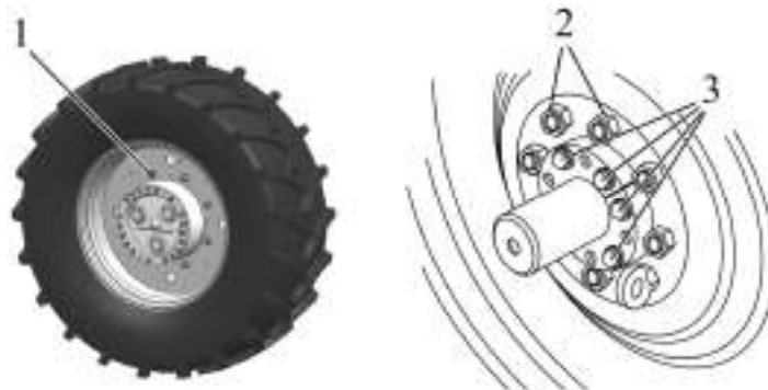
Figure 6.4.7 – Check of threaded joint torquing of wheels mounting
