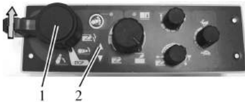
1 – handle to control lift linkage; 2 – annunciator of FLL uplift.
