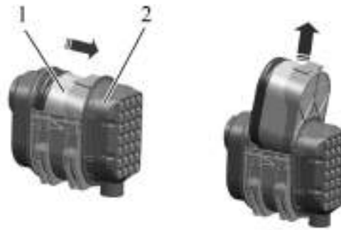
1 – main filter cartridge; 2 – integrated "multicyclone" unit.
