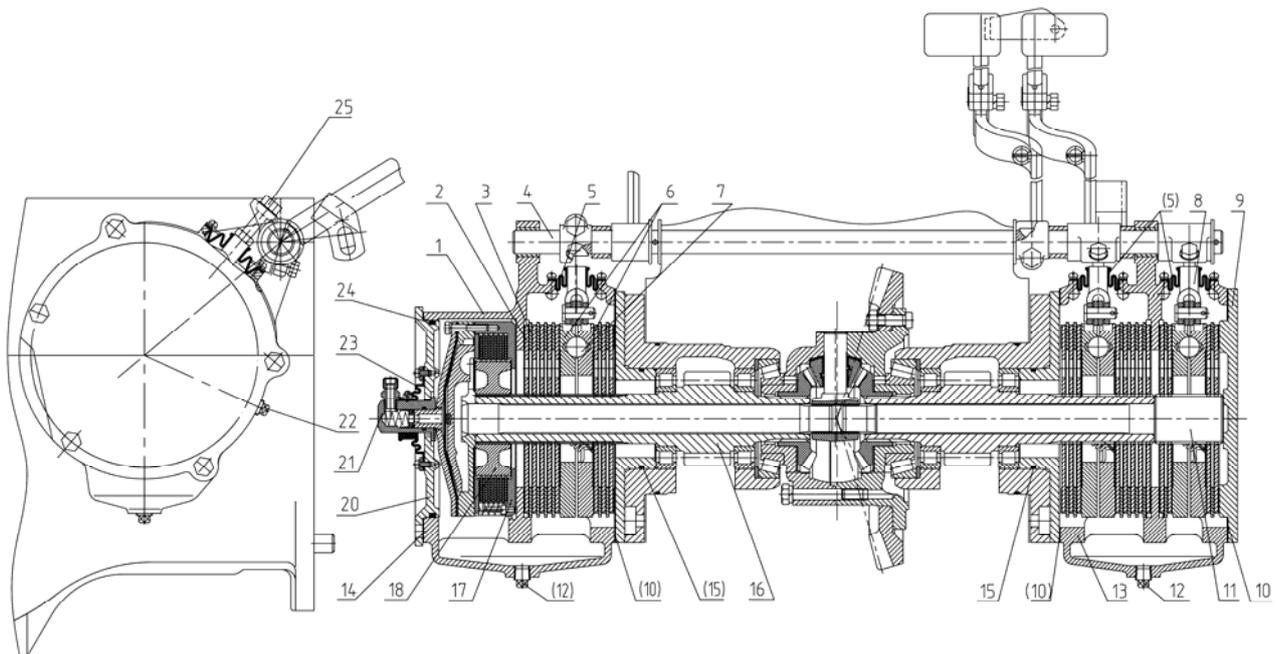
1 — body housing, 2 — friction disk, 3 — spacing disk; 4 — pedal shaft; 5 — sealing hood; 6 — pressure plate; 7 - ball. 8 — park brake, 9 — cover; 10 — gasket; 11 — park brake shaft, 12 — drain plug, 13 — brake housing; 14 — gasket; 15 — O-ring; 16 — axle drive gear; 17 — lock clutch; 18 — hub, 20 — cover; 21 — adapter; 22 — check (filler) plug; 23 — sealing hood; 24 — O-ring; 25 — adjusting bolt.
