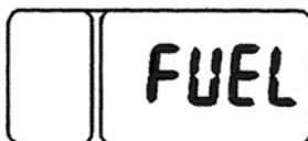
When frequency signal from FPFV is missing for 2 seconds, LCD display of ID displays “FUEL” message.
