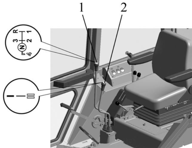
1 – gear shift lever; 2 – range selector lever
