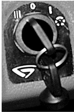
Figure 1.2 – Switch of starter and instruments
