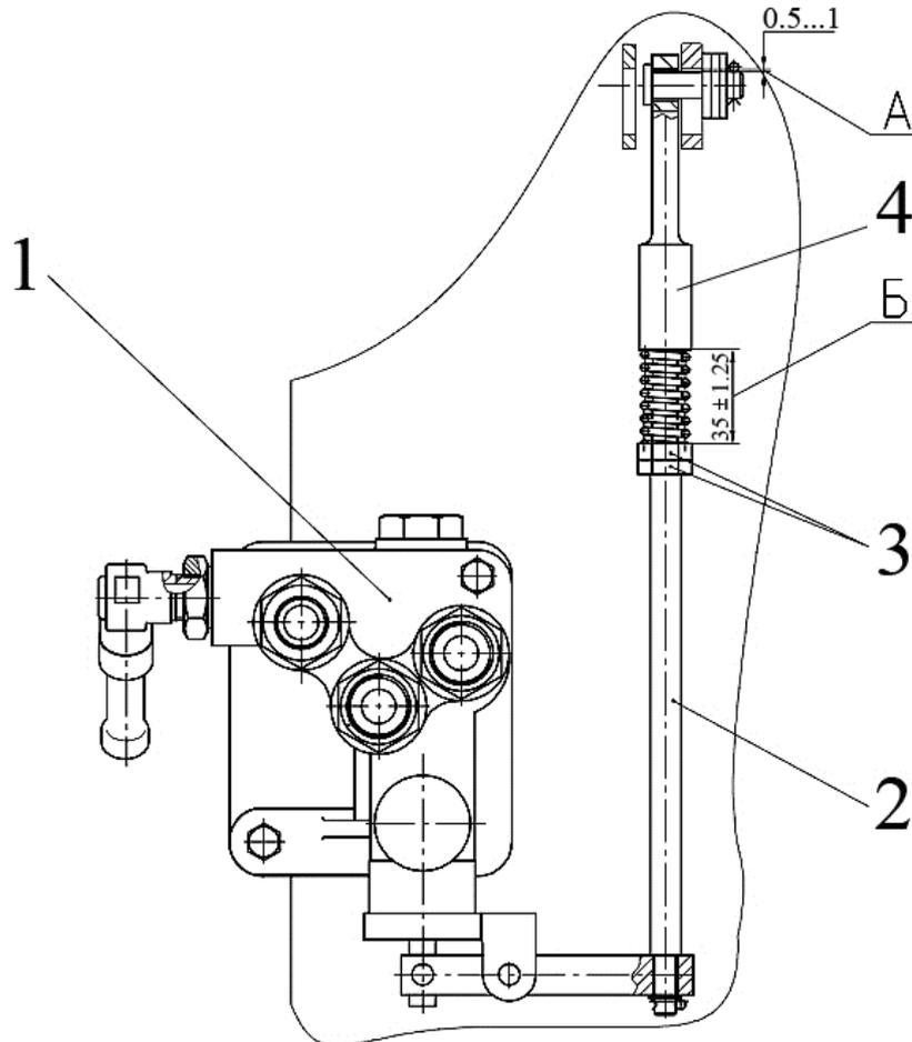
1 – brake valve; 2 – pull-rod; 3 – nut; 4 – rod end
