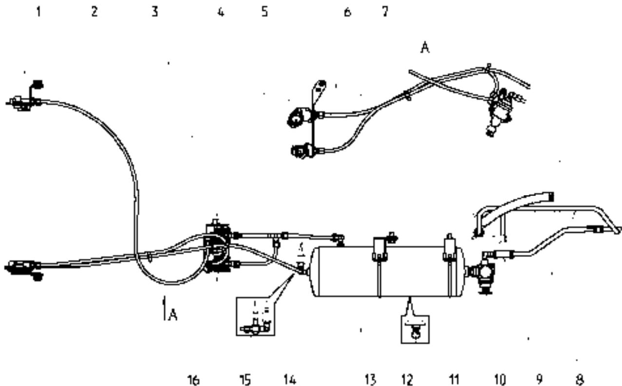
1, 4, 5 - coupling heads; 2 - control manifold; 3 - brake valve (single-wire); 6 – connecting line; 7 – supply line; 8 - line from engine intake manifold; 9 – compressor; 10 – air bleed valve; 11 - pressure regulator; 12 – condensate drain valve; 13 - cylinder; 14 - air pressure sensor; 15 - emergency air pressure sensor; 16 - brake valve (single-wire).
