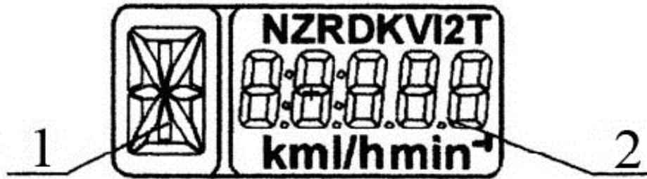
“1” – digital identification of transmission switch position (digits from 0 to 6) or letter identification of reduction unit switch position (letters L, M, H, N);
