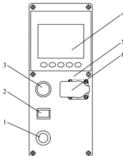
1 – diagnostics activation button switch; 2 - failure diagnostics indicator; 3 – cigarette lighter; 4 – information display; 5 -panel; 5 - appliance receptacle 12 V/ 25 A.
