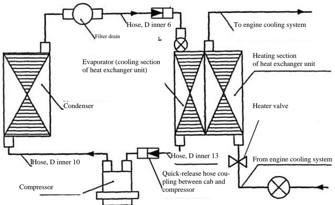
Figure 2.11 – Cab air conditioning and heating system
