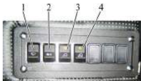
1 – windscreen wiper switch; 2 – cab heater switch; 3 – rear working lights switch; 4 – switch of front working lights on cab roof.
