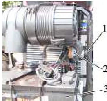
1 – button; 2 – AB manual disconnect switch; 3 – accumulator battery. Figure 2.2.3 – Installation of the accumulator battery manual disconnect switch
