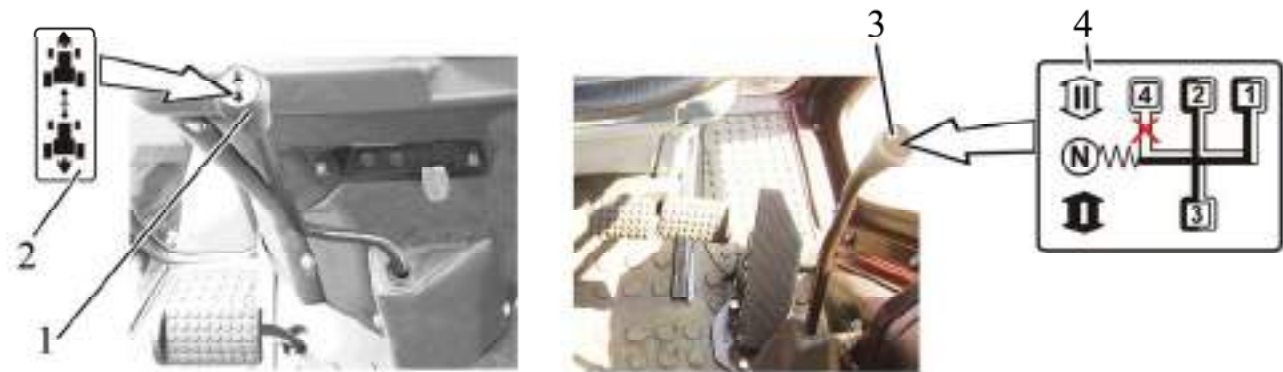
1 – control lever of the reverse gear unit; 2 – diagram of passes shifting of the reverse gear unit; 3 – lever to shift ranges and gears of the GB; 4 – diagram of GB ranges and gears shifting.
