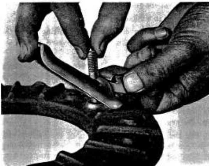
FIG. 33 REPLACING THE STRUT AND RELEASE LEVER
