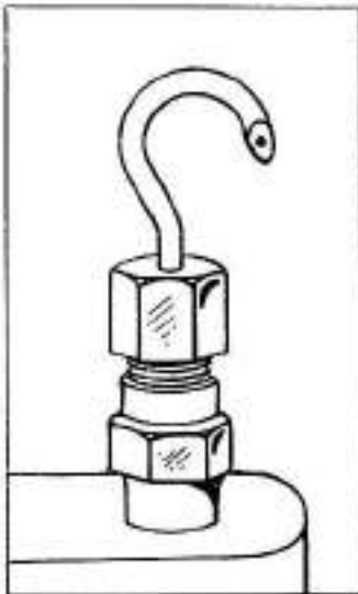
FIG. 21 SPILL PIPE FOR TIMING INJECTION PUMP
