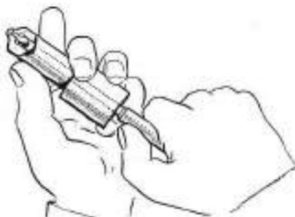
Fig. 73—Remove any carbon from dome (tip) cavity with dome cavity cleaner as shown above.
