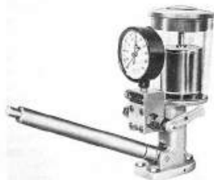
Fig. 67—An injector tester is necessary to check condition of nozzle and adjust injector pressure setting.
