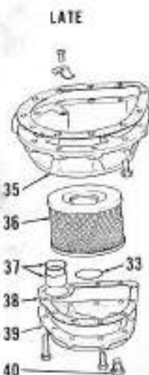
Fig. 276—Exploded view of pump suction filters and covers for early and late 1210, 1212, 1410 and 1412 models.
