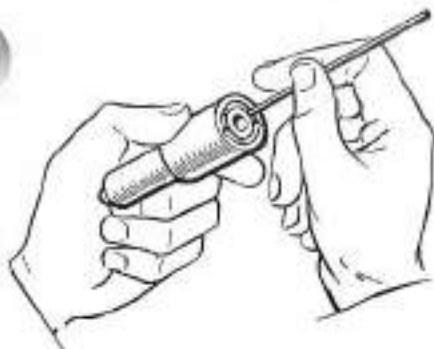
Fig. 70—Clean out small feed channel bores with drill or wire as shown. These bores are rarely choked and insertion of drill or wire by hand will be sufficient.
