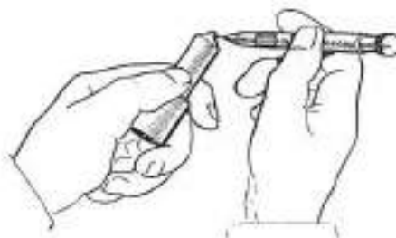
Fig. 74—Using pin vise and proper size of cleaning wire to probe all carbon from the four injection spray holes in each nozzle tip.
