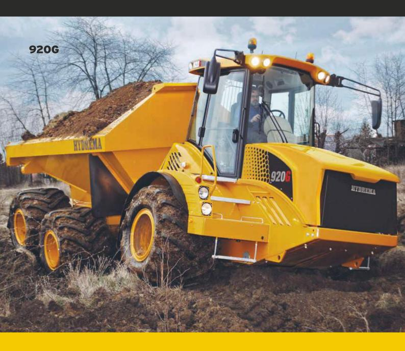
The 920G is the obvious choice for earthmoving in soft terrain. With maximum traction, better grip and record-setting low ground pressure.
