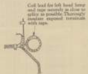
Illustration No. 14B View showing wiring when right head lamp only is installed. (Note:- parts not shown are the same as in illustration No. 14).
