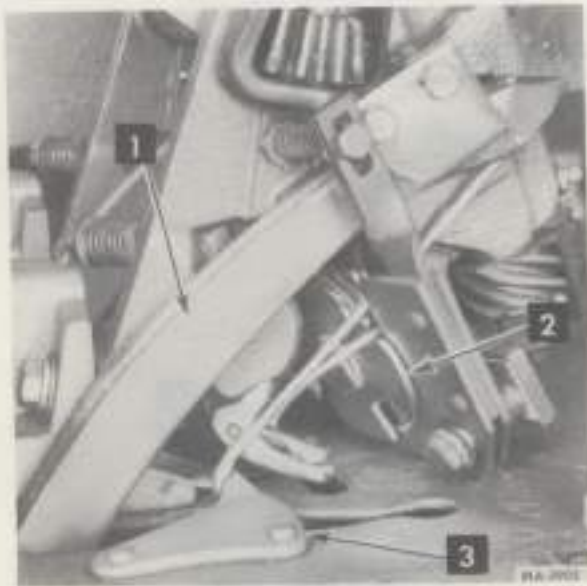
1 - Needle 2 - Disk 3 - Breast plate finger
