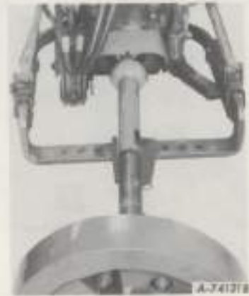
Illustr. 5B 430 Baler. Two-joint universal drive shaft.
