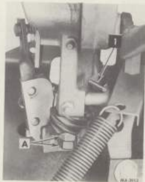
1 - Insert 3/16-inch drill or punch Illust. 26C Timing hole in knotter frame and disk.
