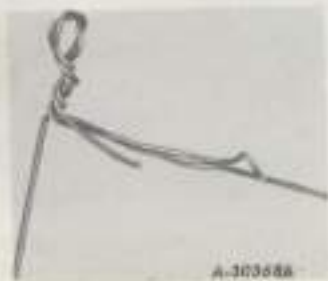
Illust. 34A Proper wire twist.
