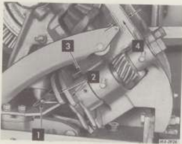
1 - Disk wire 3 - Needle wire 2 - Disks 4 - Dimension is 3/8 to 3/4-inch
