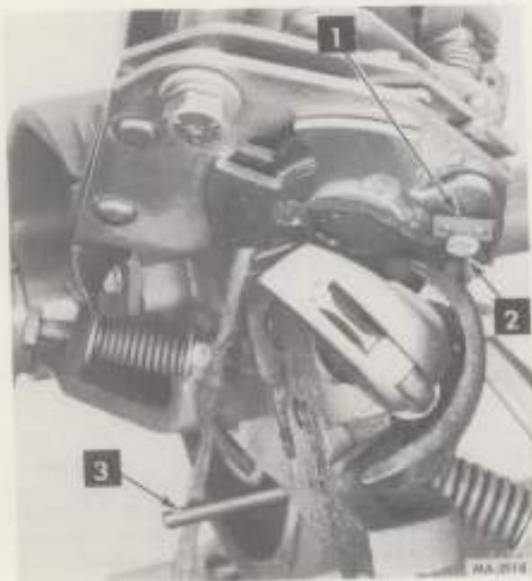
1 - Twine knife blade 2 - Twine knife blade screw 3 - Punch
