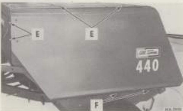
Illust. 18A Removal of auger shield end.
