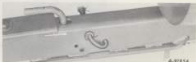
Illust. 41C Lifting jack in stored position.
