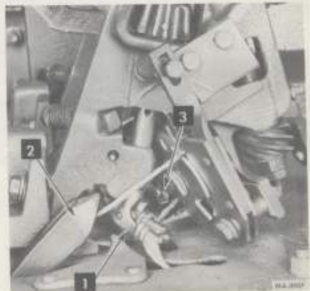
1 - Knotter hook 2 - Needle 3 - Knife
