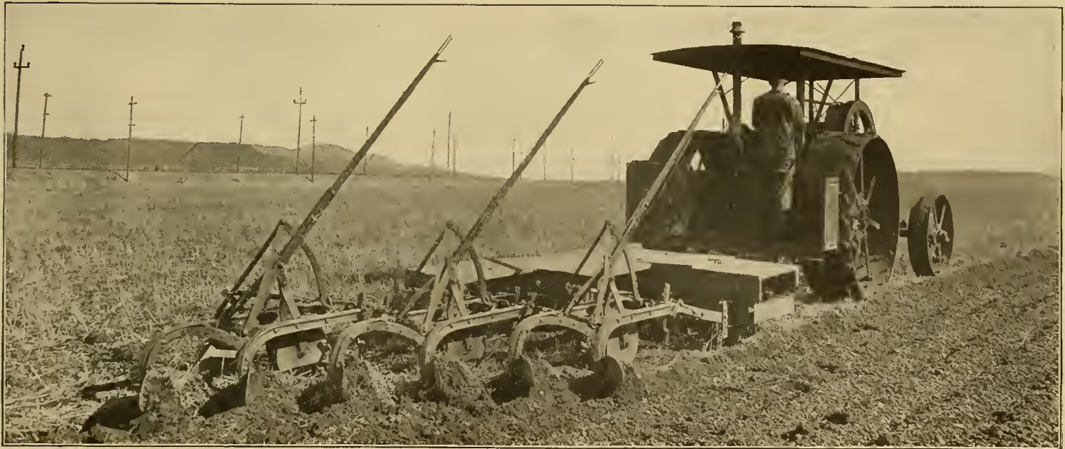
A 25-horse power I H C tractor pulling six 14-inch bottom plows. This tractor was working under favorable conditions in stubble ground
