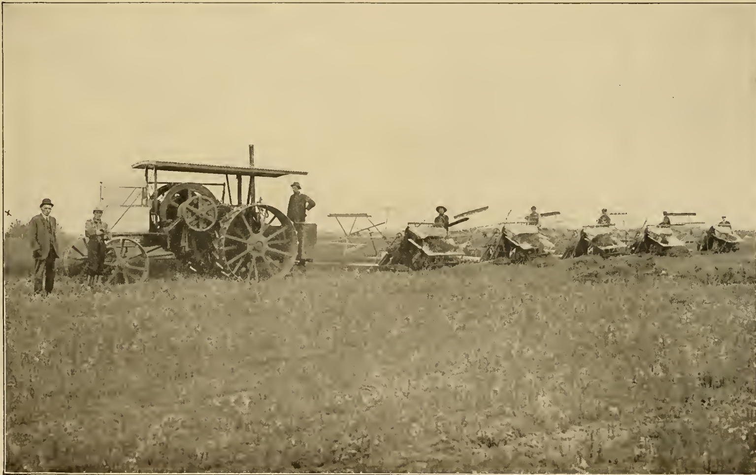
25-horse power Titan tractor, pulling five I H C binders in a flax field on the farm of John Archie McDonald, Ft. Quapple, Saskatchewan
