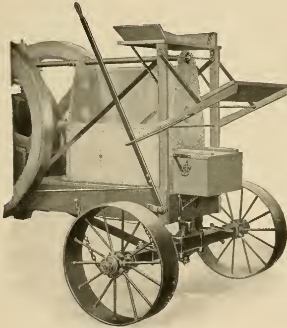
Detail of Portable Engine Showing Water Tank and Front Trucks
