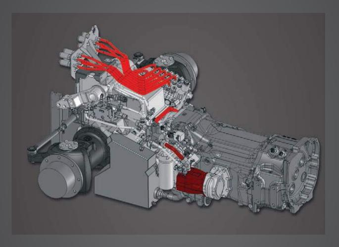
The high-performance power hydraulics from BOSCH supplies 88 l/min with the variable displacement pump.
