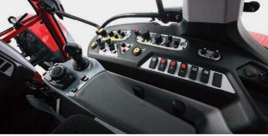
All driving functions within easy reach The most important driving functions are grouped together on the Ldrive controller: Function keys for Crawler mode, cruise control and foot throttle mode are at the front. The keys behind them activate allwheel drive and the differential.
