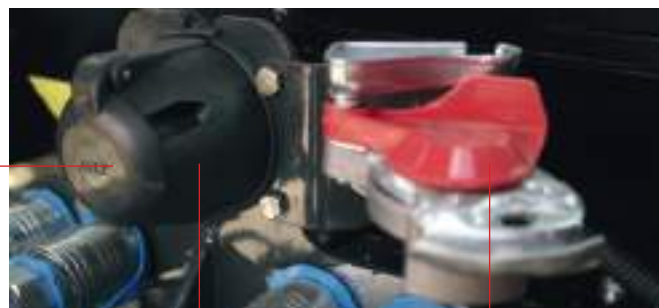
Trailer power connection plug
