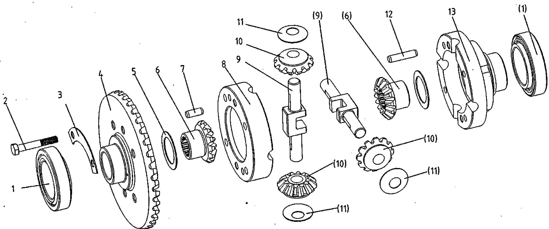
7.A.5 前驱动桥总成 (304.31.014A部件) Front Wheel Drive Axle (304.31.014A Assembly)
