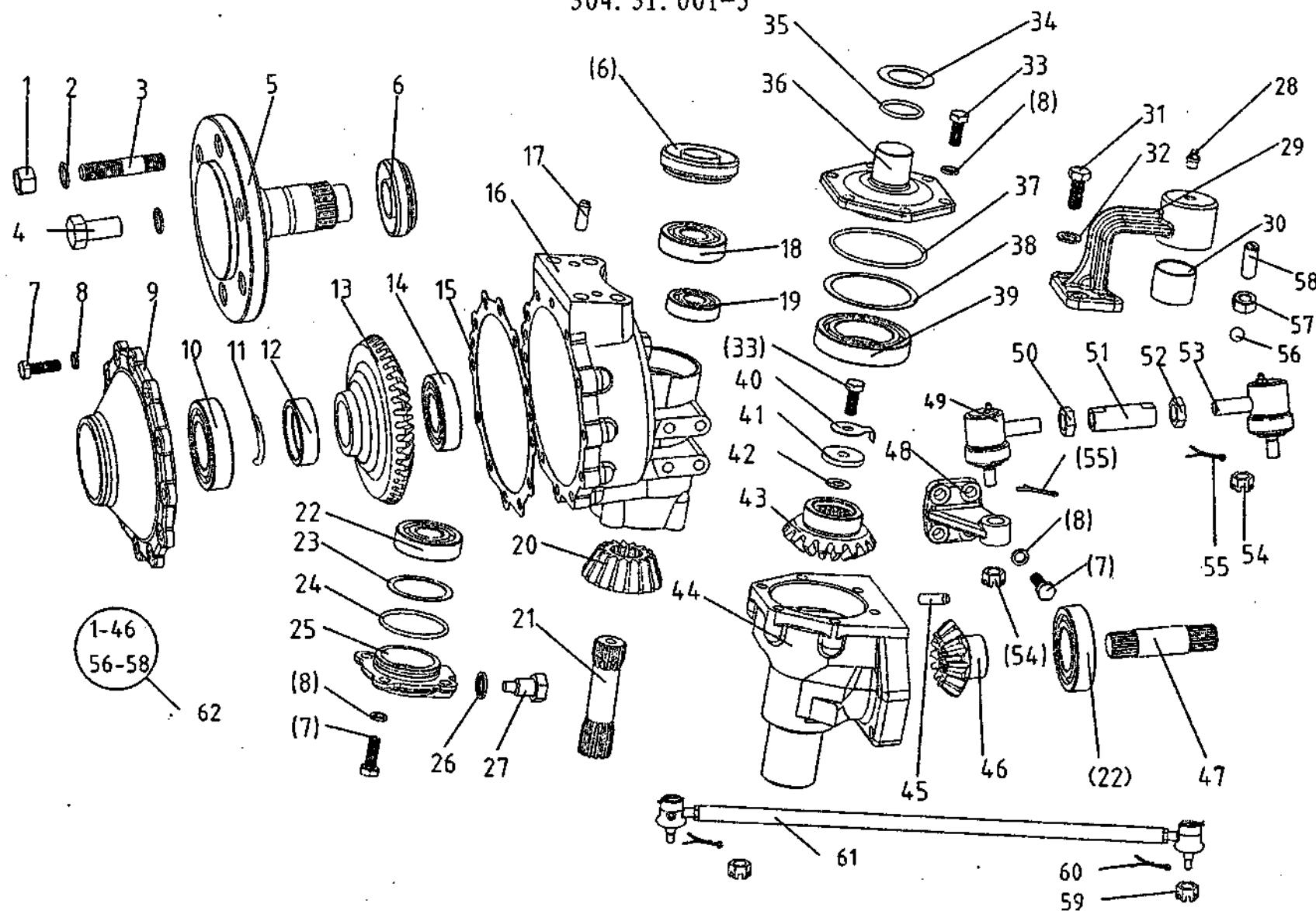
7. B. 2 前驱动桥总成 (左边减速) Front Wheel Drive Axle ( Left Side-Slowdown )
