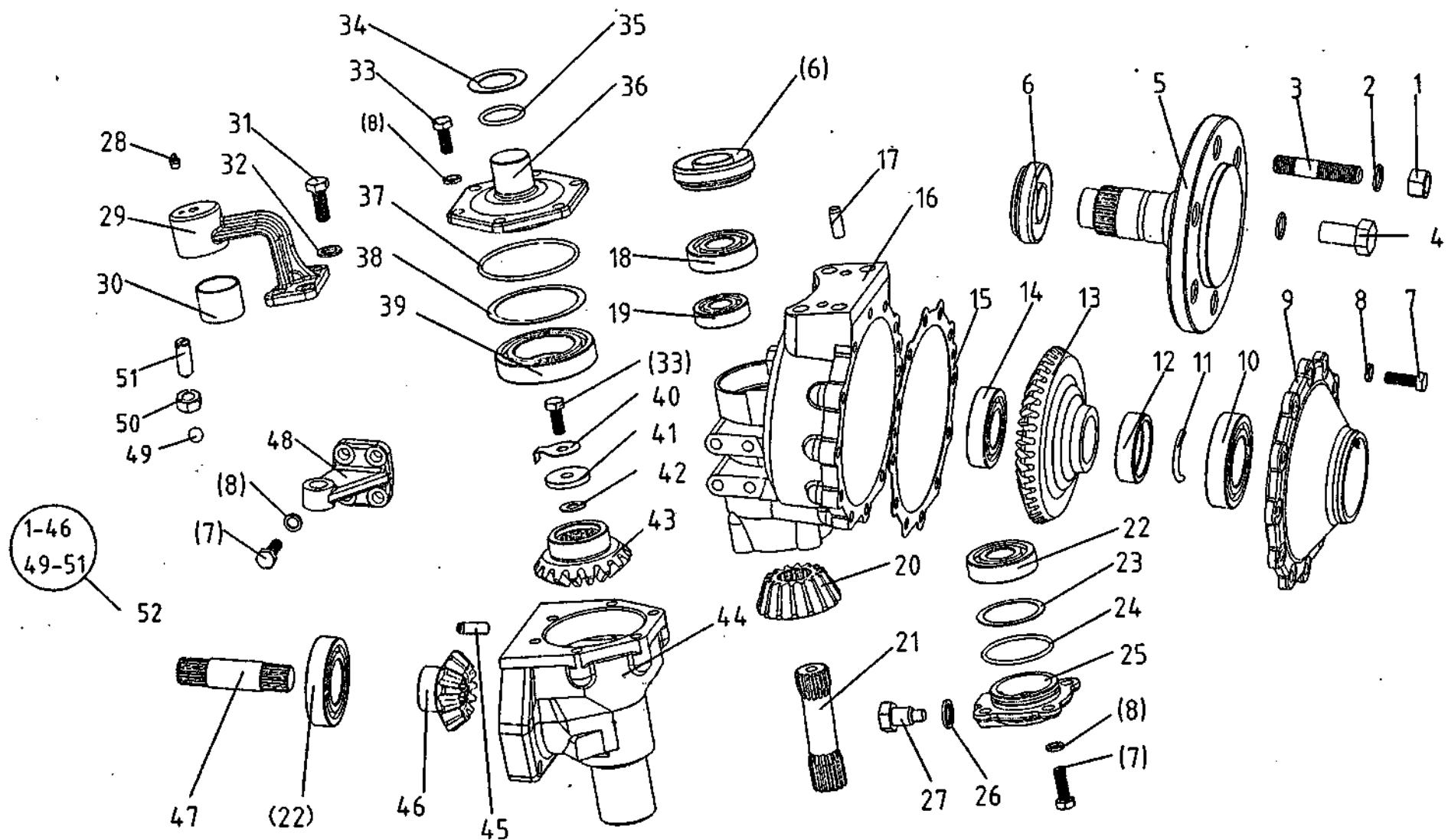
7. A. 3 前驱动桥总成 (右边减速) Front Wheel Drive Axle ( Right Side-Slowdown )
