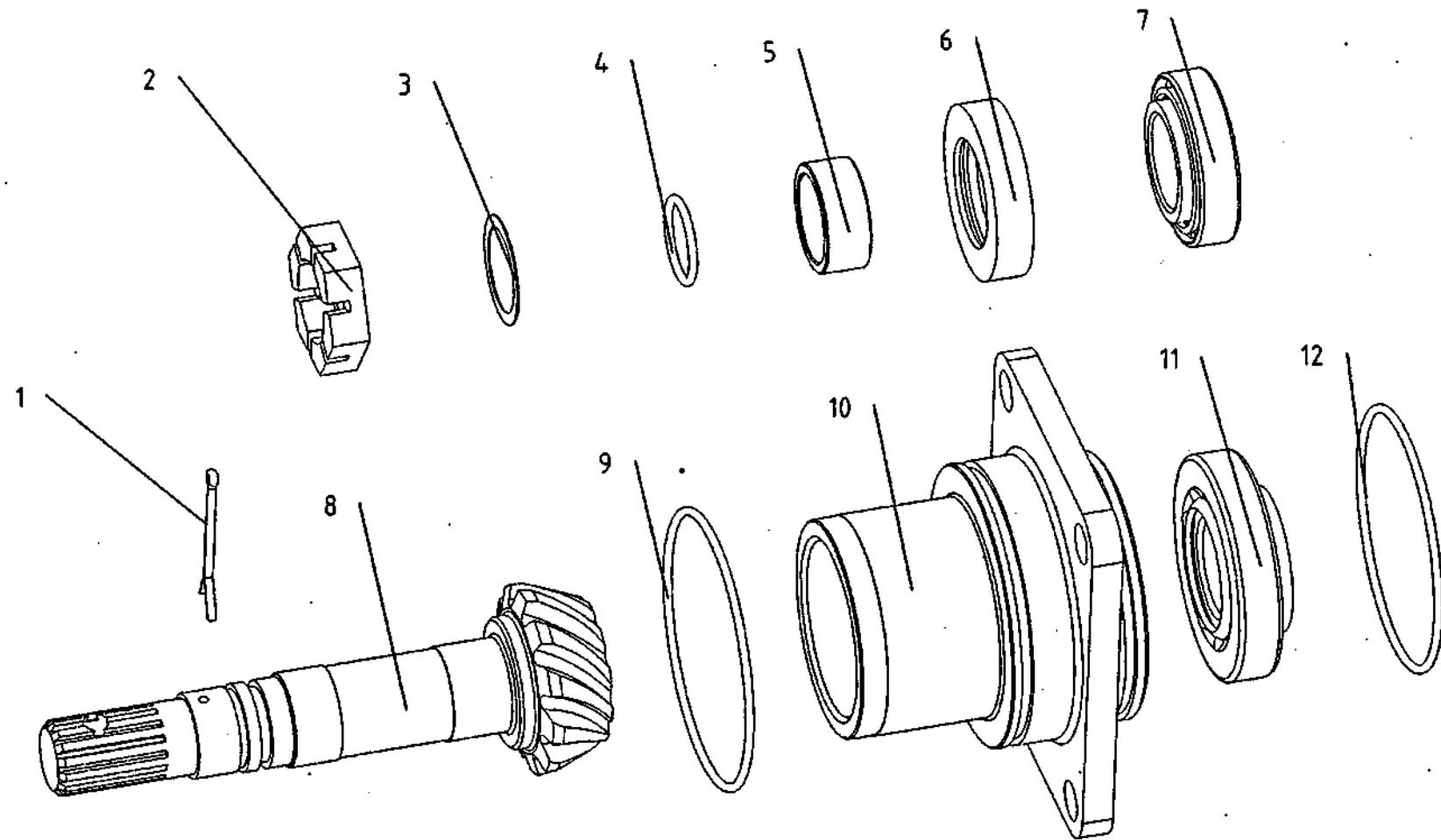
7. A. 4 前驱动桥总成 (304.31.022-1部件) Front Wheel Drive Axle (304.31.022-1 Assembly)
