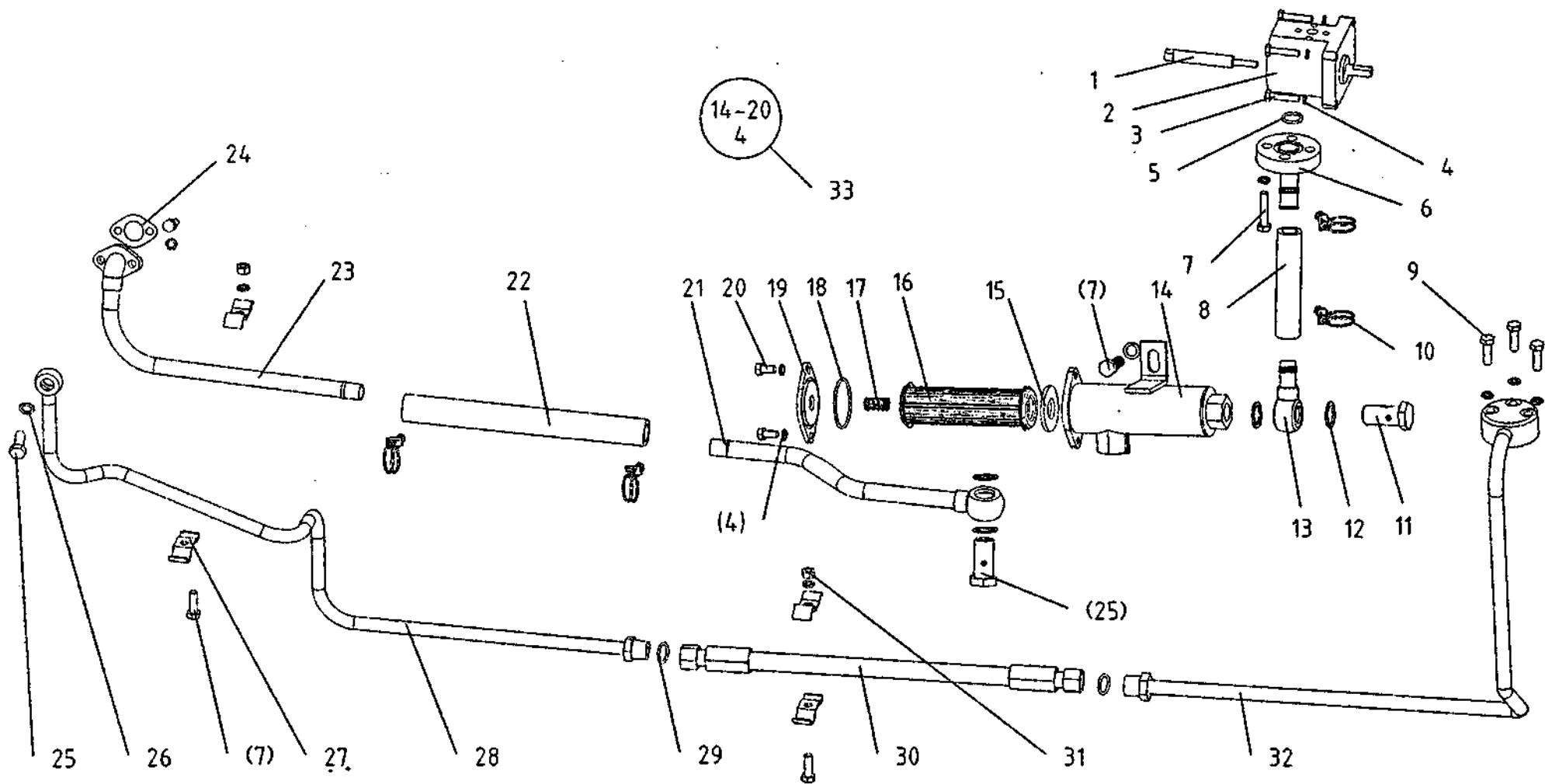
28. A 油泵、滤油器、油管总成 Oil Pump, Filter, Pipe and Fittings
