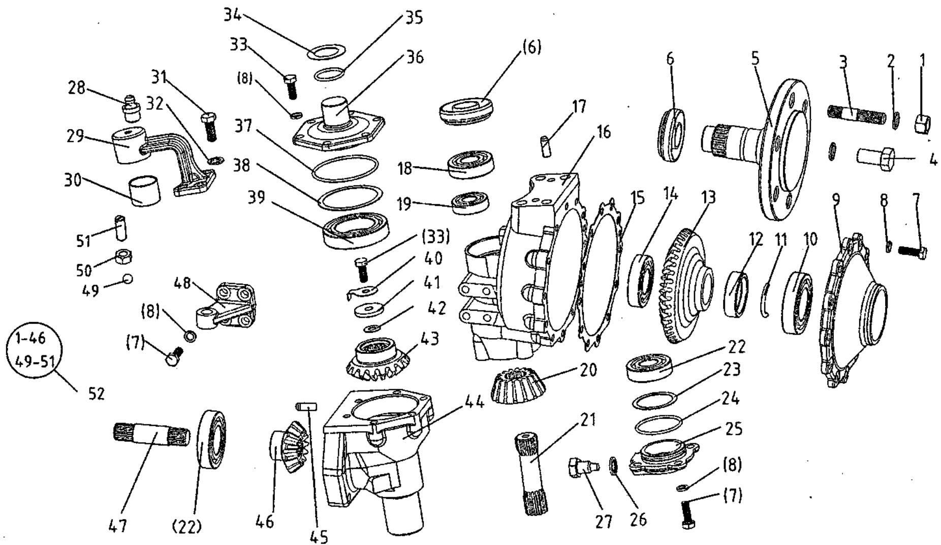
7. B. 3 前驱动桥总成 (左边减速) Front Wheel Drive Axle ( Left Side-Slowdown )
