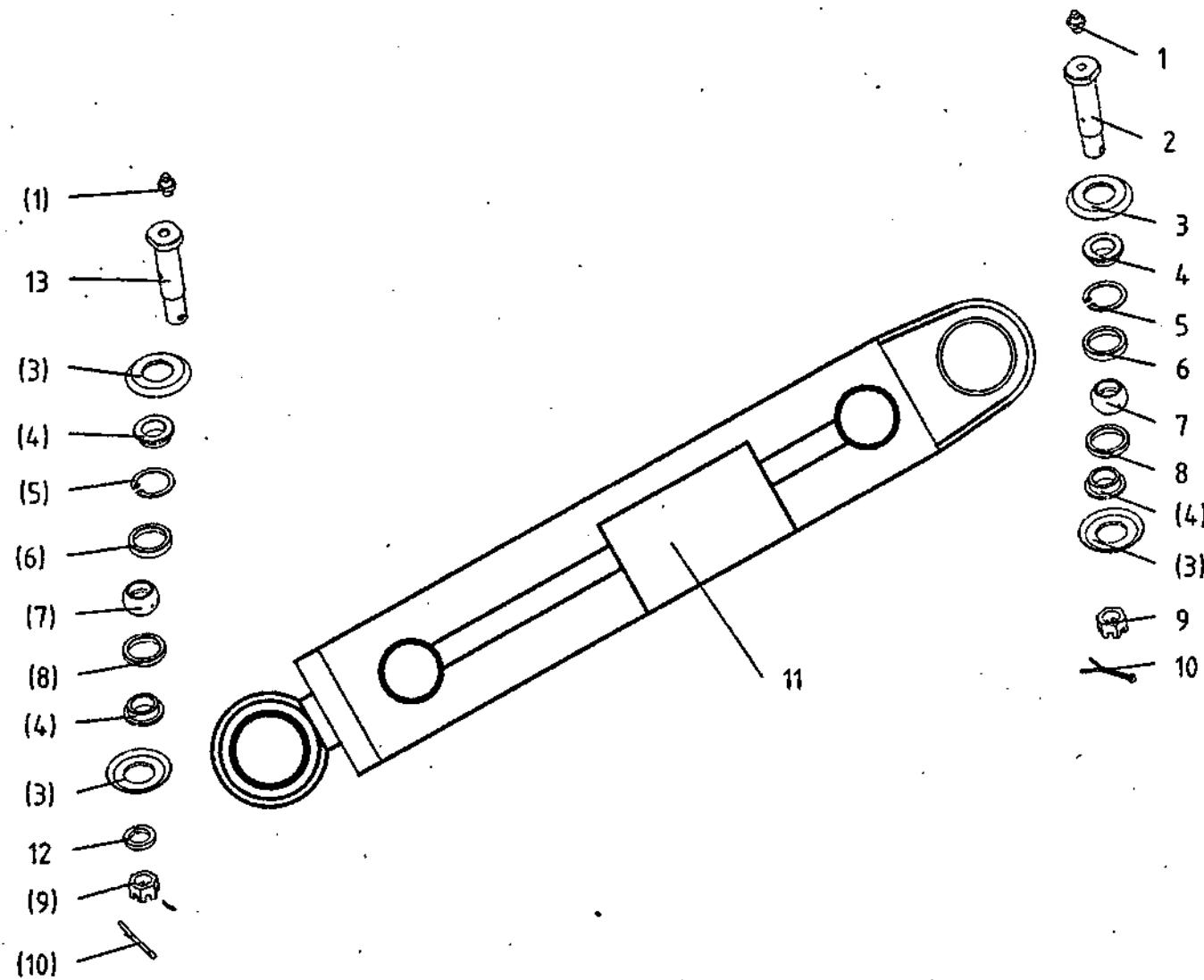
15.2.A 油缸拉杆总成Cylinder Rod Assembly
