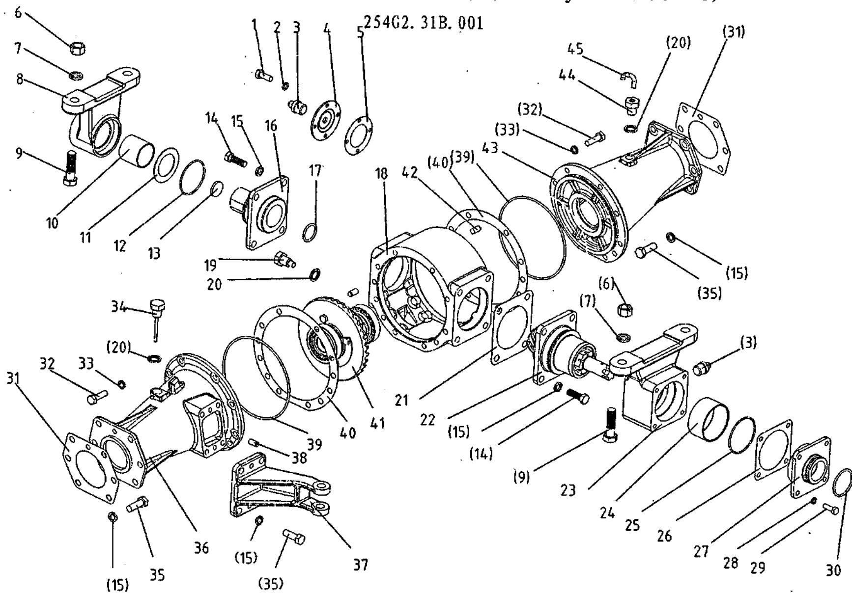
7. A. 1 前驱动桥总成(中) Front Wheel Drive Axle (Middle) (for Tire 6.00-16)
