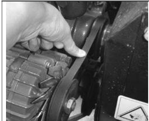
Figure 4-21 Fan Belt Tightening Adjustment
