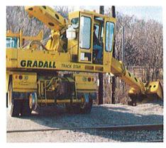
Track Star incorporates the Gradall 5-way boom...lifting, digging, tilting, swinging and telescoping with simultaneous movements of the boom improving cycle time. A variety of attachments permit you to perform a wide range of jobs with one machine. A unique Slide-A-Boom is included in the Track Star package. This unique feature adds 3' to the boom length
