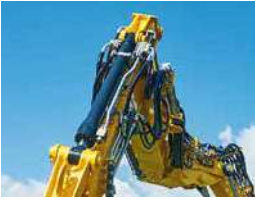
Two-piece offset boom to increase working performance
